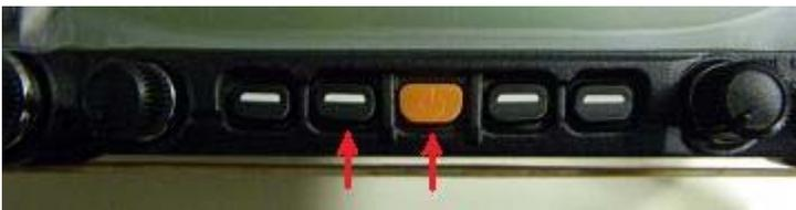
Turn the FTM-350 on while pressing and holding the key, which is located to the left of the power switch.
