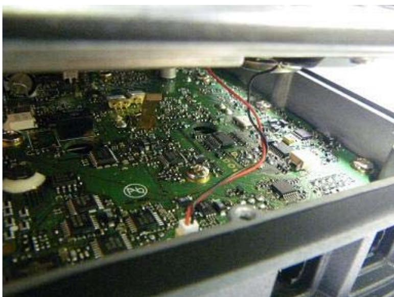
Connect the 2-pin connector from the speaker to the connector on the MAIN Unit, and then affix the Top Cover to the FTM-350.
