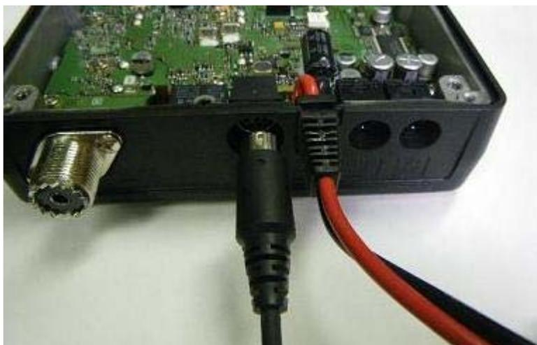
Disconnect the programming cable from the FTM-350.
