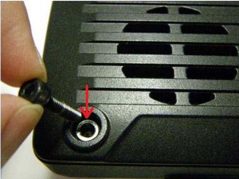
Place a screw, with spring washer, into each of the four screw holes in the top cover.
