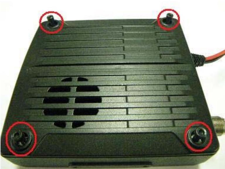
Tighten each of the four screws. (This procedure requires a 3.0mm Hex wrench.)
