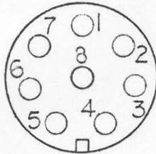
If the rotor control cable plugs are wired pin to pin ("1" to "1", "2" to "2", "3" to "3" etc.) the cable will be correct.
