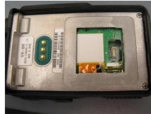
3. Locate the only resistor visible on the board, just to the left of the Bluetooth plug and carefully remove it:
