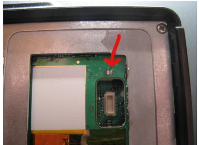
4. Clean off ALL the residual adhesive and put on a new (supplied) adhesive cover. This is important to preserve the waterproof seal!
