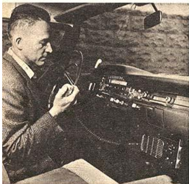
Mason shows off one of his SSB CB units mounted for mobile operation. Set draws about 42 watts.
