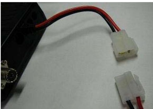
Turn The Power Switch OFF and remove the power cable from the FTM-350.
