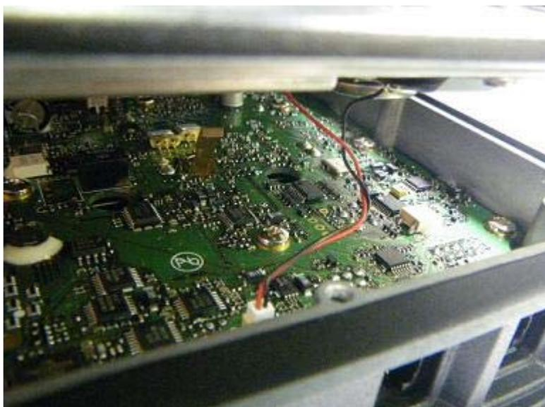
Carefully lift and move the FTM-350 Top Cover to access the Program Switch.
