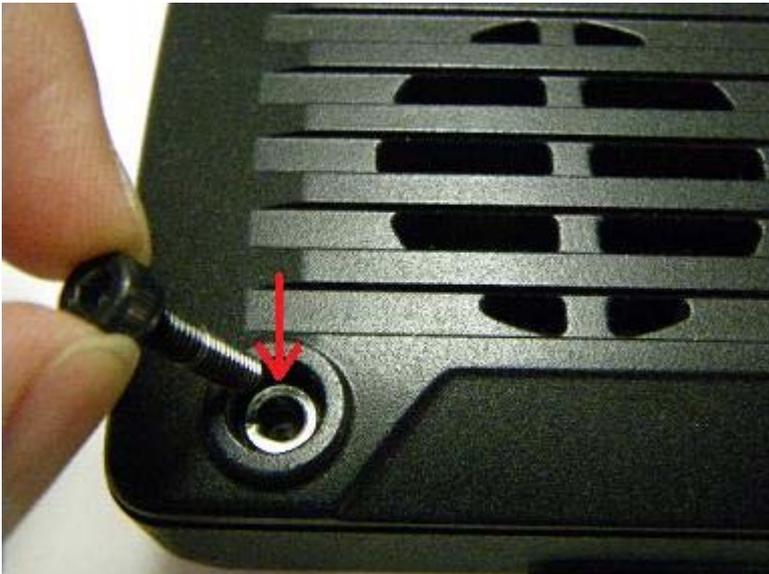
Be careful; do not lose the four spring washers that are used with the four screws.
