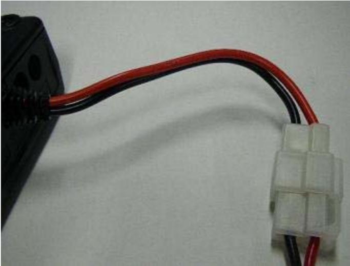
Connect the 13.8V DC power cable to the FTM-350.
