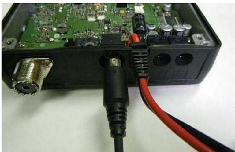
Connect the CT-140 or CT-142 programming cable to the DATA jack (Mini-DIN connector) on the back panel of the FTM-350.
