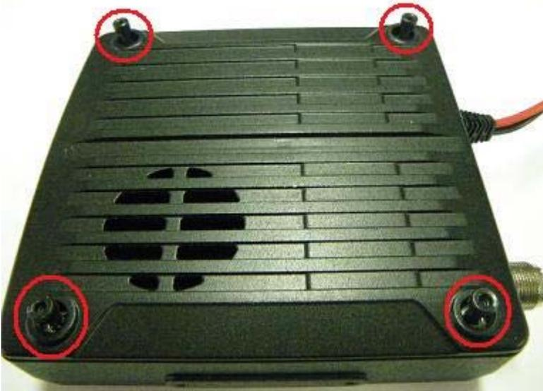
To remove the FTM-350 top cover, remove the four screws.
