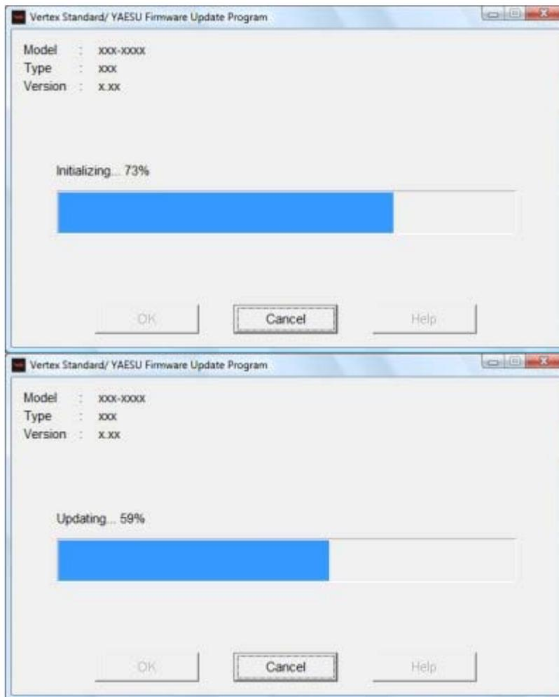
When the [OK] button is pressed, the initialization sequence completes and then the firmware is updated. Wait until the updating is complete.(It takes approximately **4 minutes**.)
