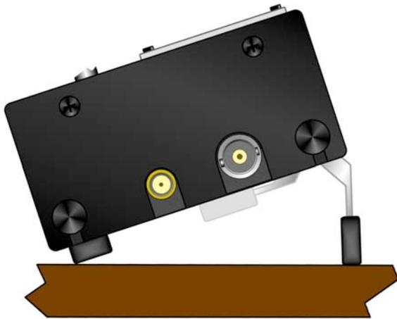
**⚠ DO NOT unplug the cable joining the two large printed circuit boards except as instructed during kit assembly or option installation. The cabinet can be opened up and laid flat for battery change, leaving the cable connected.**
