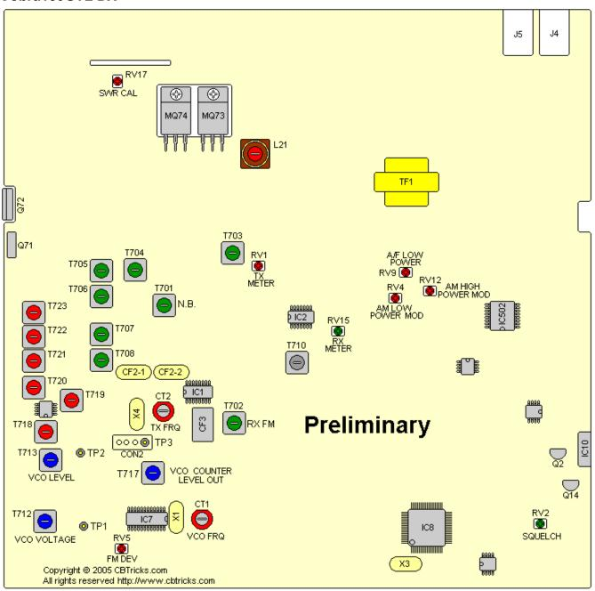
A description of all circuits and devices provided for determining and stabilizing frequency: Frequency (from 28.000mhz to 29.695mhz) of transmitting, as receiving, frequencies are provided by PLL (phase locked loop) circuitry. The purpose of the PLL is to provide a multiple number of frequencies from VCO (voltage controlled oscillator) with quartz crystal accuracy and stability from one crystal oscillator reference frequency.
