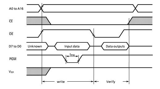
Note1: When  $V_{cc}$  power supply is turned on or after,  $V_{pp}$  must be increased. When  $V_{cc}$  power supply is turned off or before,  $V_{pp}$  must be increased.
