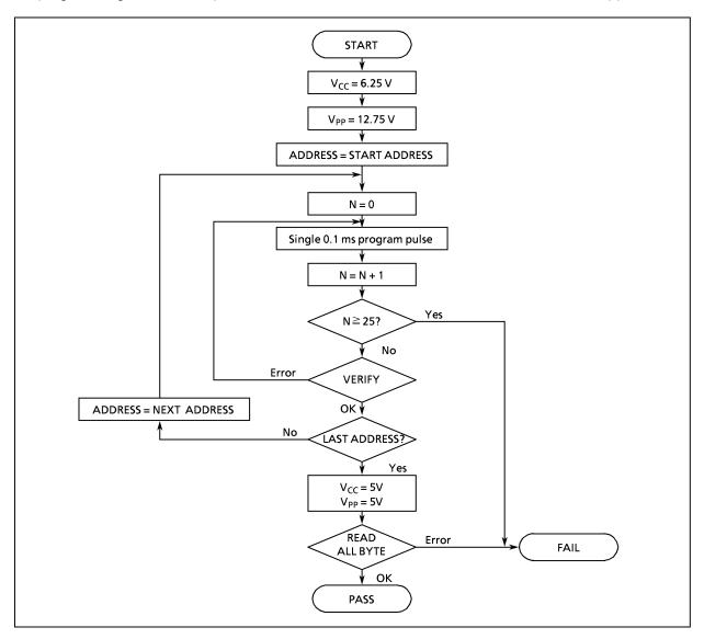
Figure 1-4. Flowchart of High-speed Programming
