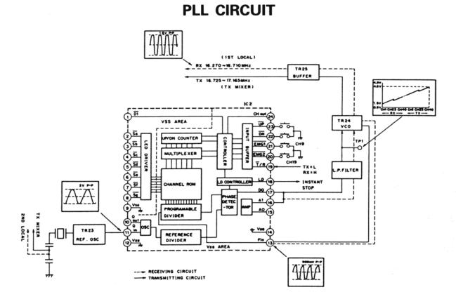
The VCO is an oscillator which controls oscillation frequency in accordance with input voltage change. The VCO output is mixed with a signal in the transmitter or receiver circuitry. A portion of the VCO freguency is fed to IC2 (1/N divider).
